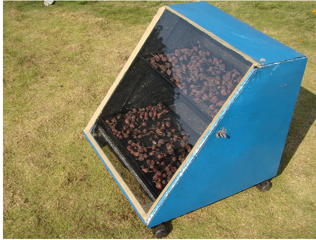
FIG. 2. Closed view of solar dryer for drying of large cardamom.
